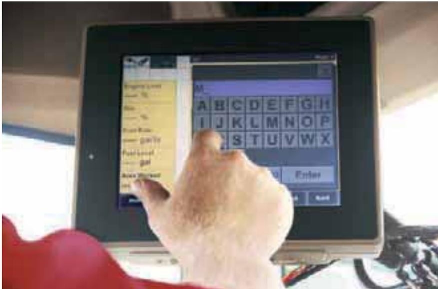
► **The AFS Field Performer** can be equipped in your new Case IH Puma, Magnum, Steiger, and QUADTRAC tractors and Axial-Flow 7010 & 8010 combines. It allows the operator to record and log fuel usage, individual operator performance, acres per hour, and engine efficiencies.
